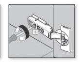
Door depth adjustment: Rotate rear spiral tech cam screw #3 to adjust door gap (+3mm,-2 mm).
